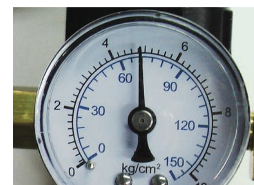
9. IMPORTANT: Set the regulator pressure to 70psi/4.85 bars or performance may be degraded.
