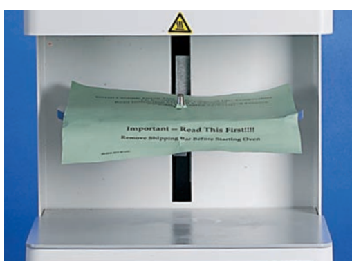
7. Turn on the furnace, wait for table to come down, then remove green paper.
