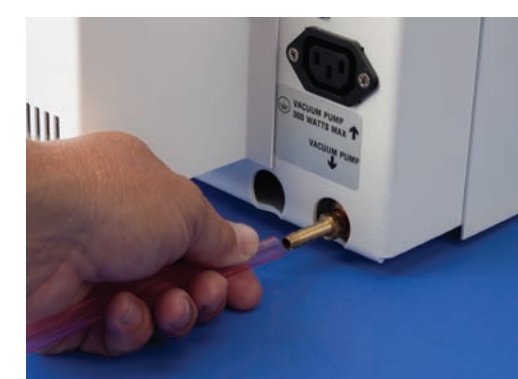
5. Remove black cap using needle nose pliers and attach the 1/4" pink vacuum hose from the pump.
