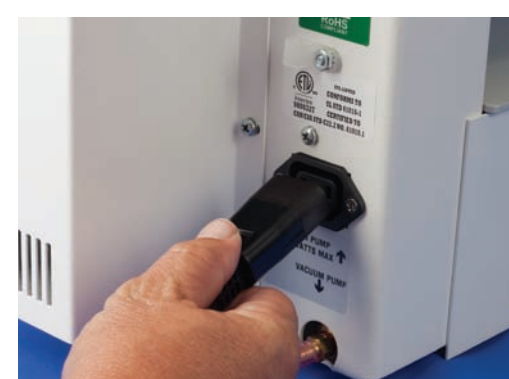
4. If you have a Whip Mix pump, plug it directly into the furnace outlet.
