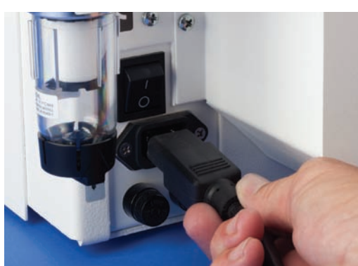
3. Install the power cord and plug into a dedicated grounded outlet.
