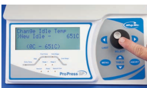
3. Turn the Select knob to change the temperature to 651°C. Select.
