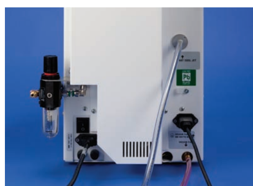
6. If Quick Cool connection is desired, 1. Remove the brass hose barb from the furnace accessory box. 2. Remove the muffler from the output end of the vacuum pump. (The input and output valves are identified by arrow indicators on the vacuum pump near the inlet or outlet.) 3. Install the brass barb to output end of the vacuum pump (where the muffler used to be). 4. There should be two hoses included; one in the accessory box, the other inside the vacuum pump box. Use the clear hose included in the accessory box for the Quick Cool Air Jet.
