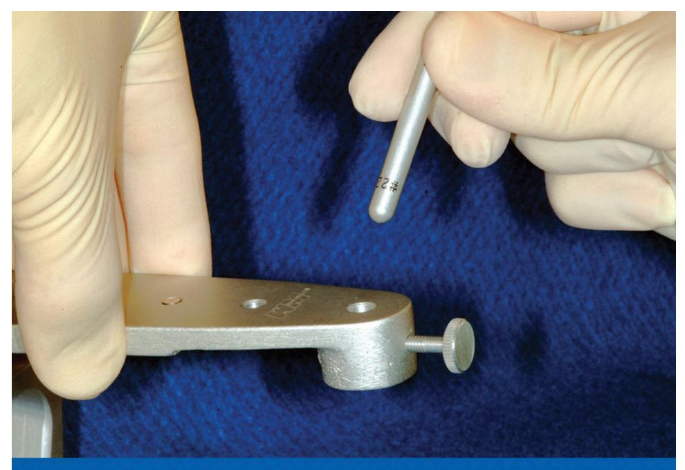
Loosen the #8511 incisal guide pin screw and remove the incisal guide pin.
