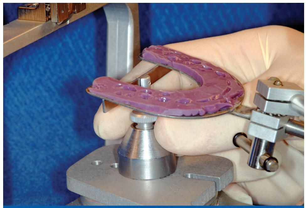
If using the face-bow fork support, raise it until it touches the undersurface of the face-bow fork.
