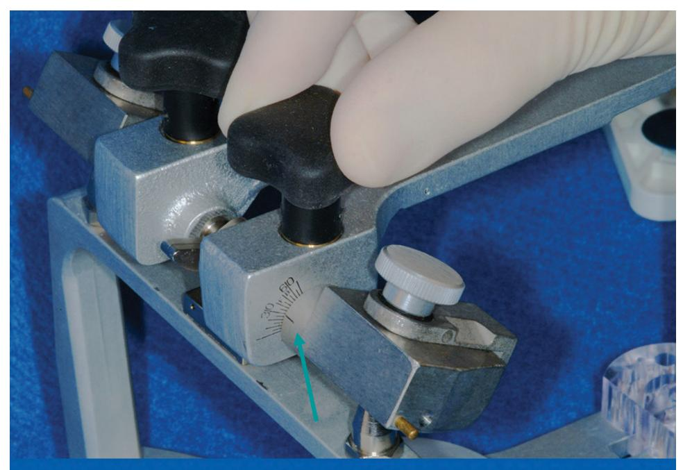
If using the Model #2340, set the condylar inclination to the  $30^{\circ}$  mark.
