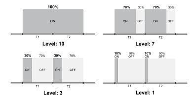
**NOTE:** For the best results curing a small print, we strongly recommend using a lower intensity output and a longer curing time.
