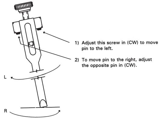
9. When adjustment is obtained, pin is on center web. Tighten to top knob.
