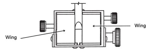
7. Pin should rest on center web and not on a wing of the T6 Table.
