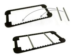
Universal Build Plate Jig / Metal Rods: To clean printed parts while they are attached to the printer build plate, place the Metal Rods (two of them) into the appropriate slots of the Universal Jig (adjustable positioning to fit build plate size up to 180mm × 90mm) (7.08" × 3.54").
